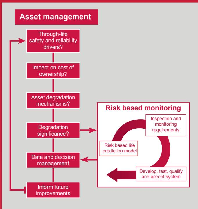
The fundamental premise here is that the 'through-life safety and reliability drivers' are identified and understood. The sensitivities to cost and the degradation mechanisms affecting these drivers also need to be understood. It is then possible to predict how the plant will degrade over time and therefore define an inspection regime to maintain safety and reliability.
