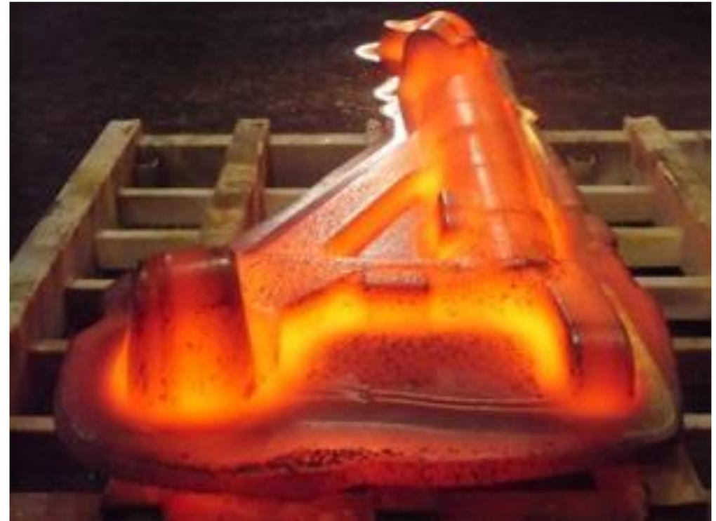
Forged CRES main fitting after closed die operation. (Courtesy of Aubert & Duval)
