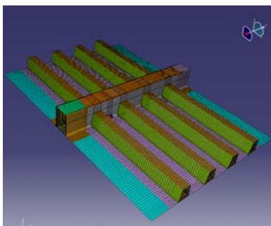
Figure 1: Transverse Frame Structural Model
