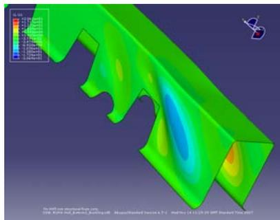
Figure 2: Transverse Frame Shear Web Skin Wrinkling
